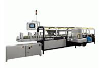
ARPAC's TrayStar® tray loaders are capable of reaching speeds up to 70 trays per minute. These continuous and intermittent motion machines are designed for a wide range of products including cans, bottles and boxes. Every TrayStar® system is easily integrated with other equipment, including tray turners/stackers and shrink wrappers.
