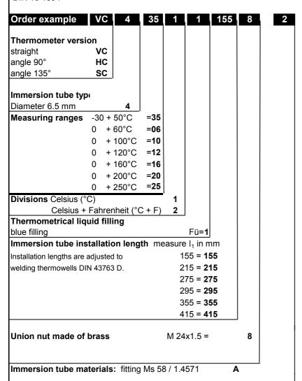
We deliver the thermometers of the type series "4" generally with a steel tube diameter 6.5 mm on the capillary lower part, suitable in thermowells with orifice 7 mm to protect the glass and to avoid that glass parts fall into the orifice of the welding cover when the capillaries break.
