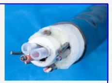
Extractive CEMS umbilical using high efficiency aerogel thermal insulation.
