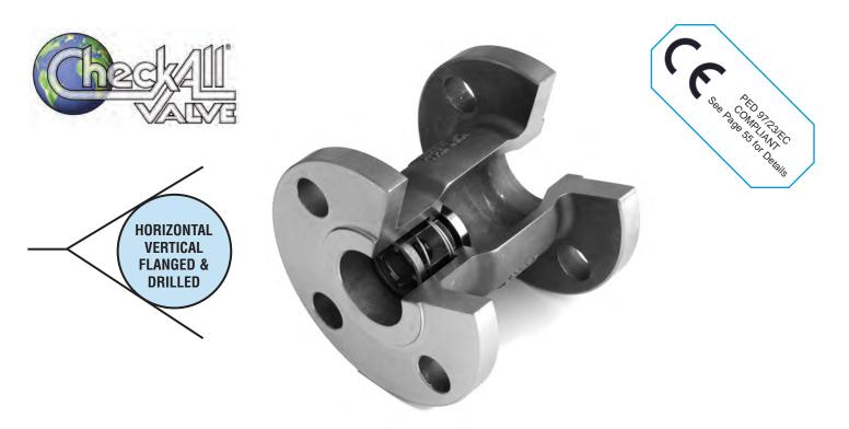
The **Check-All**<sup>®</sup> **Flanged & Drilled (HV)** check valve is a one piece cast body valve with ASME/ANSI B16.5 Class 150 flanged ends. The HV series valve is used when higher flow rates and lower pressure drops are required. The valve is available in sizes 1 inch through 10 inches and standard materials of CF8M (cast 316 stainless) and WCB/WCC (cast carbon steel). The HV series valve is designed for use with mating ANSI class 150 flanges. Other materials are available upon request.
