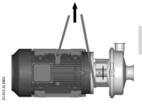
ATTENTION! Always remove the motor shroud before hoisting.
