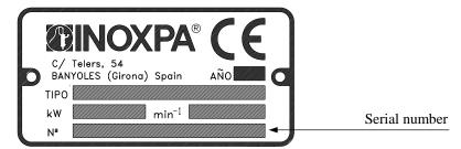
Figure 3.1: Characteristics plate.
