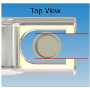
Releasing the clamp is only possible when the wing-nut has been significantly loosened to enable the smaller diameter of the eyebolt to swing and pass through the sectioned gate, this ensures the clamp cannot be knocked or accidentally opened. Complete wing-nut removal is not necessary to open the clamp since the design guarantees the eyebolt cannot swing open while the clamping union is subjected to either clamping forces or internal pressures.
