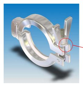
The 'gate' style section combined with the stepped eyebolt assures the clamp's bolting mechanism cannot swing open while the clamping union is part or fully assembled.
