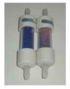
The moisture indicator (left) will alert you to when the Magnum-600 requires regeneration. The indicator on the left is blue which means that the air is very dry, and suitable for ozone generation. The indicator on the right is purple/pink, which means the Magnum-600 must be regenerated. The indicator does not need to be regenerated. It will revert to a blue color once the air from a regenerated Magnum-600 passes through it.
