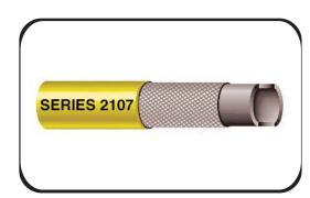
This hose is designed for applications requiring a premium quality, multi-purpose hose with superior abrasion resistance for air, oil, and some chemical applications. Excellent durability for extra long life in these applications: mining, air drill, construction, poultry plants, and other severe service. Meets MSHA requirements for flame resistant and non-conductive (1/4" - 1-1/4").
