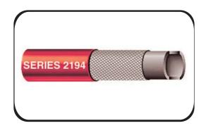
A premium quality, multi-purpose hose with excellent flexibility and maximum resistance to air, water, petroleum oils, and lubricating oils. Approved for breathing applications such as supplied air respirators. The non-conductive construction has a minimum one megohm resistance per inch at 1000 volts DC.
