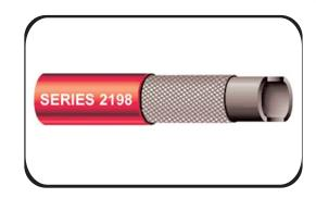
Economical and versatile general purpose hose. Excellent for air and water service as well as many agricultural chemicals including Lasso® herbicide. EPDM tube and cover resists heat, sunlight, ozone and weathering. This hose exceeds ARPM Class C oil resistance requirements. Suitable for applications such as oil mist lubricating air lines, but NOT suitable for the transfer of petroleum products.
