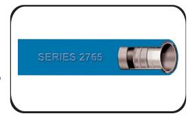
This premium hose is designed to handle water suitable for drinking in all industrial applications. The specially compounded chlorobutyl tube will not impart taste. The added features of the monofilament helix enhances vacuum rating, and the crush and kink resistance. Meets FDA, 3-A, and USDA requirements.
