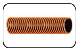
Gasoline tank truck gravity drop hose. Designed to be lightweight, tough, durable and flexible. Specially designed to handle unleaded gasoline, diesel and up to 15% gasohol. It is rated up to 40% aromatic content.
