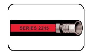
Series 2245 is designed for heavy-duty service in the transfer of petroleum products up to 50% aromatic, including leaded and unleaded gasoline, oil, and diesel fuels. Ideal for applications where an extremely lightweight, flexible hose with a high working pressure and small bend radius is required.
