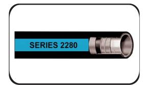
Series 2280 is a flexible, lightweight suction and discharge hose designed to handle brine, crude oil, mild chemicals, petroleum waste, sediments, sludge, slurries, and water in harsh oil field bottom sediment and waste pit recovery applications. **Do not use with refined oil or fuels.**
