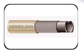
**Series 2090** is designed to evacuate hot, liquefied residue from steam cleaning operations. The high temperature, oil-resistant tube and cover withstand attack by steam vapors and petroelum-based runoff. The wire braid reinforcement provides crush-resistant durability, kink resistance and a path to conduct a static electrical charge to ground. **NOTE: Do not use for steam service.**
