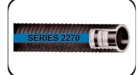
Heavy duty frac-tank hose designed to handle brine, crude oil, drilling mud, mild chemicals, petroleum waste, sediments, sludge, slurries, and water commonly found in oil field applications. Specifically designed for frac tank connections.
