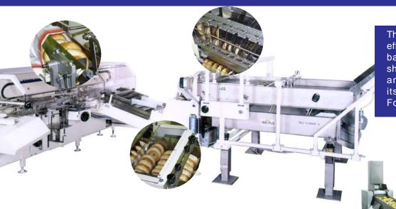
The Formost Bagel System features highly efficient aligning mechanism for bagging bagels. Feed mechanism consists of a shaker table, laning guides, drop chute, and rotary indexer. The unit deposits counted and stacked bagels into a Formost bagger bucket infeed conveyor.
