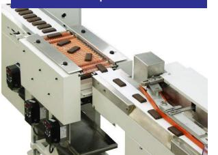
The Formost End Seal Fold Down System interfaces with a Fuji-Formost wrapper and will seal both end seals to the ends of the package. The system achieves a neat, trim, attractive package.
