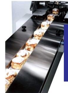
Attachless Infeed Conveyor automatically indexes soft and sticky products into a Fuji-Formost horizontal wrapper at speeds up to 120 packages per minute. Computer controlled flat belts have no lugs and are easy to remove and clean.
