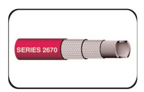
This is a heavy duty hose for high pressure water booster service on fire engines. Tube and cover compounds resist abrasion and weathering. Tough yet flexible, for resistance to flexing and surge loads. Meets NFPA 1961 requirements under current RMA specifications. Meets or exceeds UL92 requirements for 800 PSI Booster Hose.
