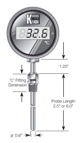
Note: For exact immersion depth, subtract length of fitting "C" from probe length
