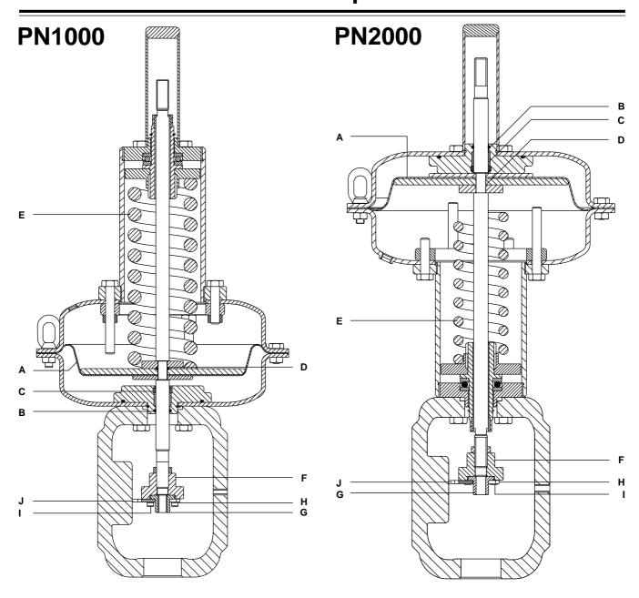
**Spare parts**The spare parts available are detailed below. No other parts are supplied as spares.
