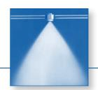
Particularly fine flat fan atomization with air or gas. Siphon principle. Internal mixing of fluids.
