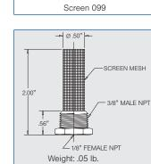
The ruby orifice produces a tightly collimated solid stream for precise, predictable cutting action. The optional strainer offers a convenient way to protect against clogging caused by stray fibers or loose bits of debris in your liquid supply.
