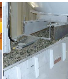
Litronic-FMS II Planar Sensor for glass manufacturing.
