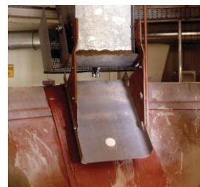
Litronic-FMS II Planar Sensor installed in a material chute.
