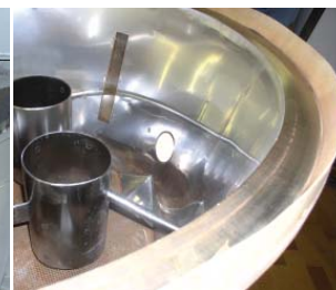
Litronic-FMS II Planar Sensor for seed manufacturing installed in a dryer.
