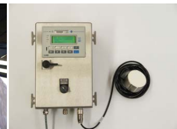
Interchange and evaluation unit and indication and parameterisation module installed in a housing made of stainless steel.
