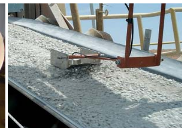
Litronic-FMS II Planar Sensor installed in a sliding shoe on a conveyor belt.
