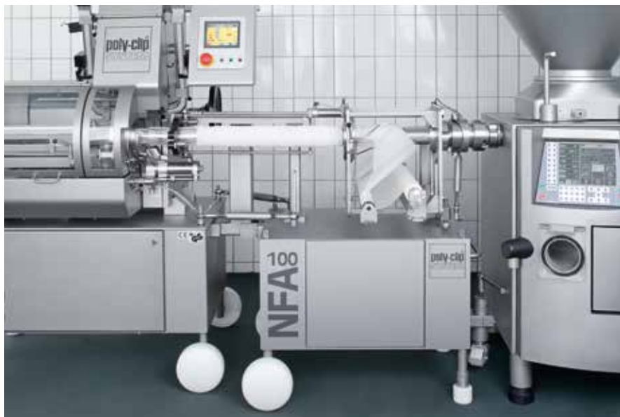
Continuous production line – NFA 100 and ICA for netted products
