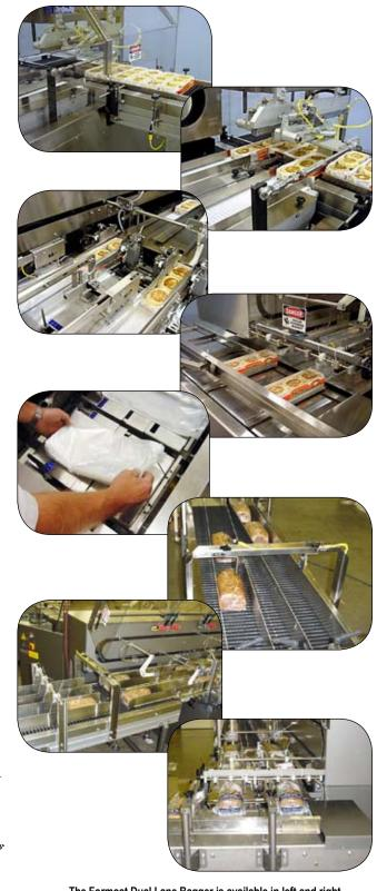
The Formost Dual Lane Bagger is available in left and right hand configurations.
