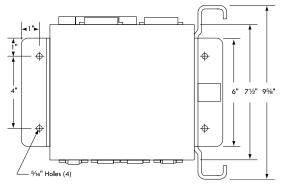
Consult the factory when certified engineering drawings are required. Dimensions shown are not suitable for construction or modifications
