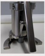
The Steinfurth Can Pressure Tester is easily ergonomic attached to beverage cans. It pierces eccentric the top lid of the can (for proper piercing outside of the pull ring area). The internal headspace can pressure can be read from the digital or analogue pressure gauge attached to the CPT piercing mechanic.
