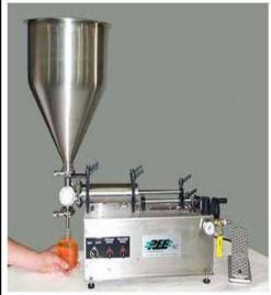
The SVS-J is our smallest piston filler, with a base of 19.5" by 9.5" and weighing approximately 35 LB.
