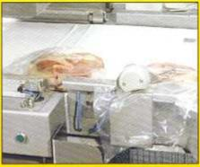
Trim Removal System (optional): Overlength of bag is cut off by rotating knives on the way into the chamber, Surplus material drops into baskets. Adjustable rotation speed suitable for all kinds of laminate bags, gusseted bags of aluminium foil and shrink bags. Does the job of both cut-off perforation and pouch piercing knives.
