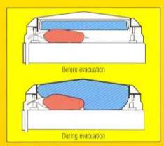
Expansion Cushion (standard) reduces evacuation time. No wrinkles on upper side of package – easier labelling. Increased production. More attractive packages – less power consumption. Snap-out Frame for easy cleaning.
