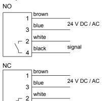
The switching outputs are self-configuring, depending on whether they are connected as PNP or NPN switches.
