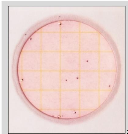
Coliform count plates are used to enumerate coliforms in 24 hours. An indicator dye in the plate colors all colonies red, and a top film traps gas (seen as bubbles) produced by the coliforms. Confirmed coliforms produce red colonies which are associated with gas bubbles. Non-coliform colonies are red but are not associated with gas bubbles.
