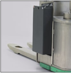
Ready for battery changing: open battery cover and removed side panel
