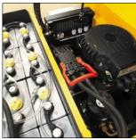
Drive and lift motor with 3-phase AC technology
