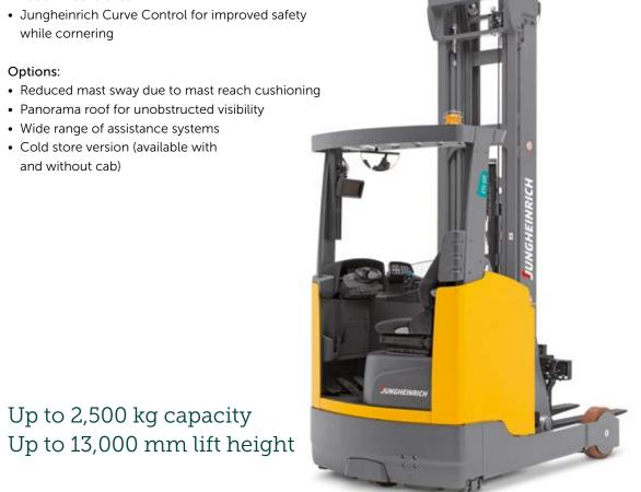
In addition to a number of lift heights and capacity classes, the Jungheinrich reach truck range also offers trucks for different ground conditions. The C Series really comes into its own when it is used for combined warehouse and yard operation. Its superelastic tyres and high ground clearance enable it to be used both on smooth concrete floors in the warehouse and on bumpy asphalt when loading and unloading HGVs, for example.
