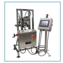
T4000-FS Force System. All stainless steel construction and highly sensitive pressure detection make it the perfect solution for testing low pressure PET bottles.
