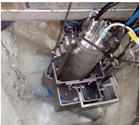
OPTIQUAD-WW installed in an open channel
