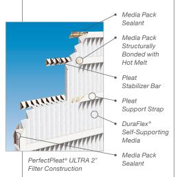
The PerfectPleat ULTRA filter is designed to consistently increase efficiency throughout the service life of the filter. The PerfectPleat ULTRA filter has approximately 25% more media than our standard capacity filter and also incorporates an antimicrobial.
