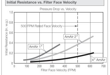
Filters are rated at 500 FPM filter face velocity. Recommended final resistance for all AmAir/CE filters is 1 in. w.g.
