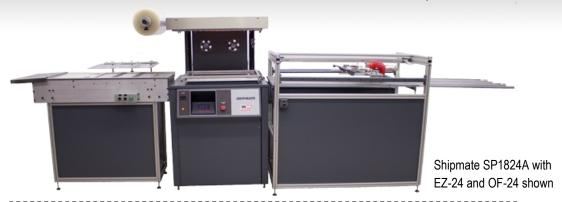
This skin packaging system is made up of three components: an automatic infeed, the Shipmate skin packaging machine, and an automatic outfeed.
